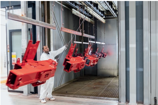
The primer and powder coating are cured in two ovens at 190 to 200°C for a maximum of 30 minutes.
