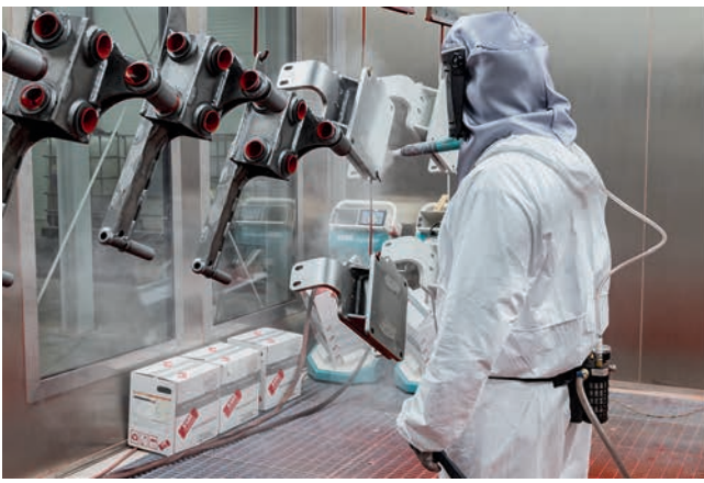
The primer (left) and the top coat are applied manually in a walk-in booth
