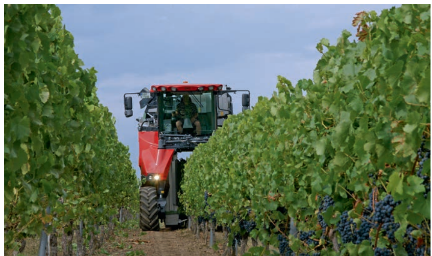
The self-driving grape harvesters are exposed to tartaric acid from the grapes and to other chemicals and therefore require very good corrosion protection.
